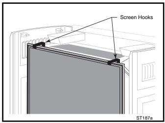
Fig. 6 Lift screen from firebox.
